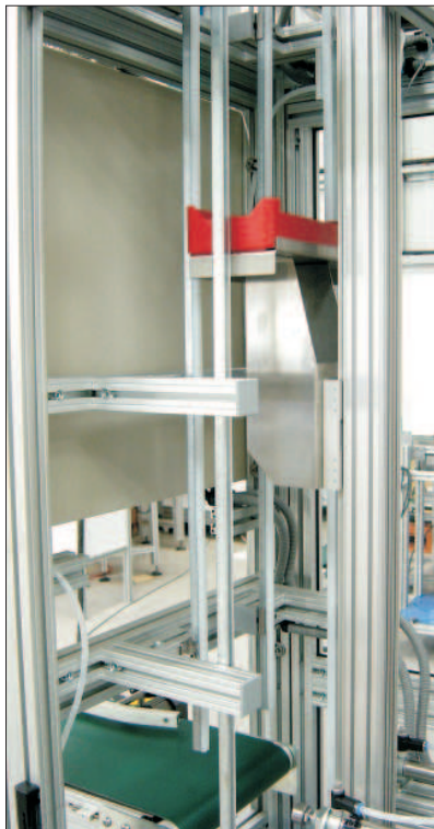
A single lift being used to transfer component carrier trays from a stores on a mezzanine floor to the ground floor of a factory
