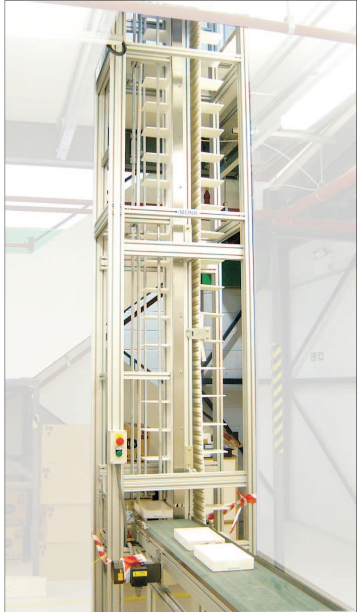
A continuous lift being installed in a stores area. Items are placed on a conveyor and form a queue, they are then automatically transferred to the floor above and escaped onto a second conveyor.
